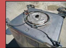
Old, Time-Consuming Nut and Bolt Hold Down Ring
