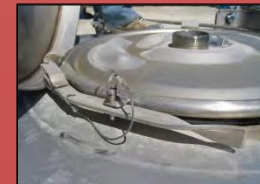
Quick-release-lever hold downing NO TOOLS REQUIRED
