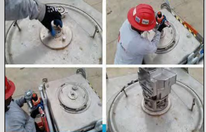
Easy and Safe Drive Unit Installation
